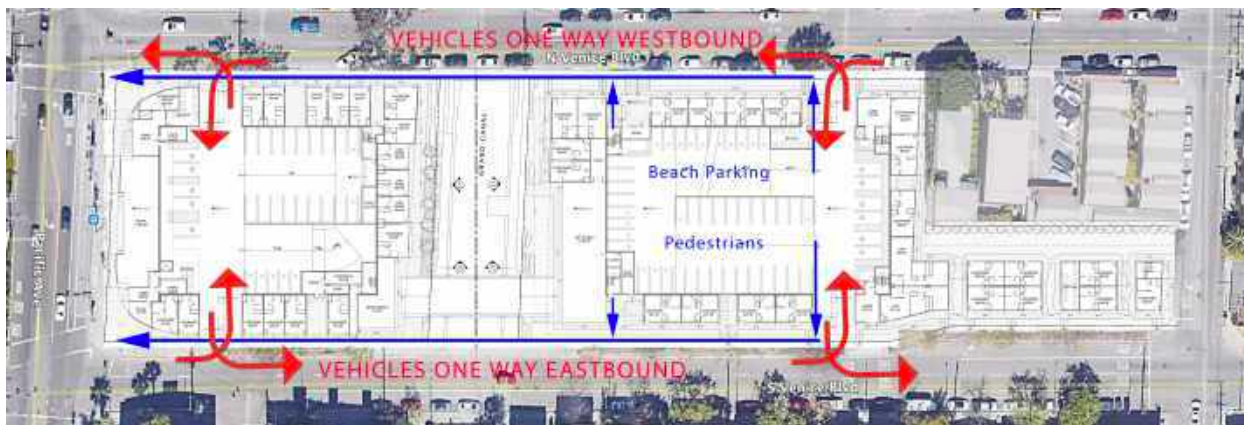
FIGURE 19 – UNSAFE PROJECT VEHICLE/VEHICLE AND PEDESTRIAN/VEHICLE MOVEMENT CONFLICTS
